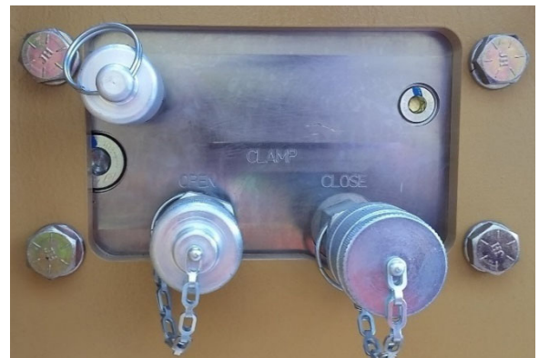
Power Unit quick disconnects, OPEN on left and CLOSE on right.
