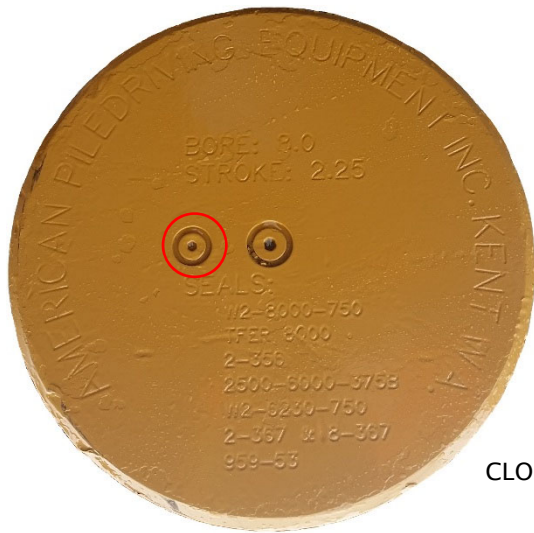
Thermal relief indicated by 2 nd off-center plug on clamp bucket face
