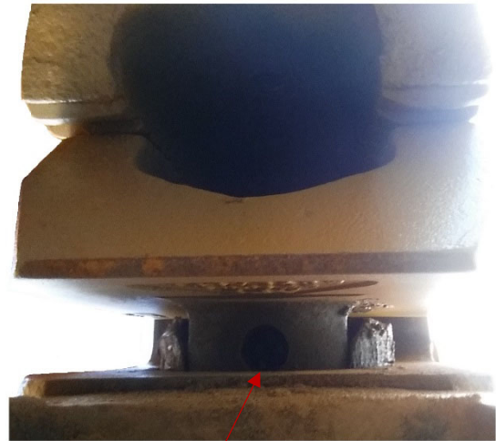
Bottom view of roll pin hole on moveable jaw.
